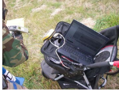
Figure 5: RAT with GPS and ADM300 on jogging stroller during first experiment
