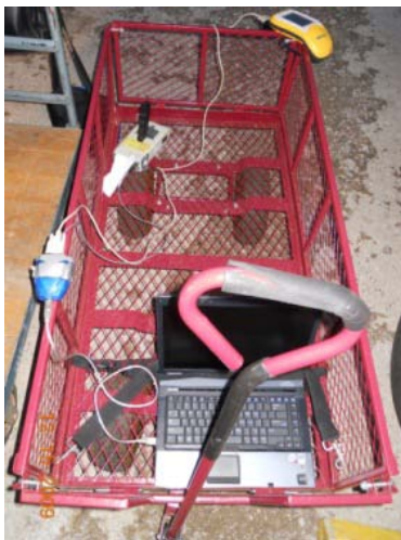
Figure 6: RAT with GPS and ADM300 on survey cart during second experiment
